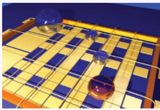
Figure 1: A digital microfluidic system (Berthier, 2018). Figure 2: A multiplex lab-on-a-chip device (Maxwell, 2016).
