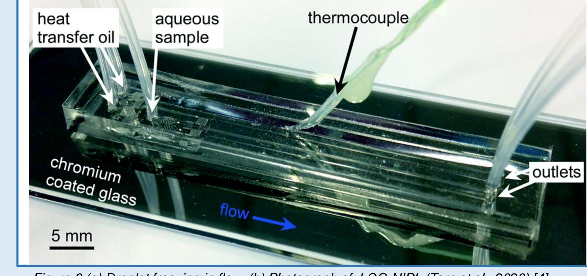
Figure 6 (a) Droplet freezing in flow. (b) Photograph of LOC-NIPI. (Tarn et al., 2020) [4]
