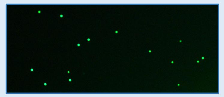
*Figure 5 Fluorescence micrograph of 2 micron particles* collected by the ESP
