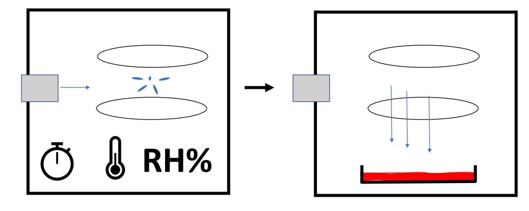
Bioaerosol of reproducible size are dispensed into the CELEBS chamber, where they are caught between two electrodes in an electrodynamic trap. Here they are subject to tight control of temperature and humidity, before deposition into cell tissue growth media ahead of downstream infectivity assay.
