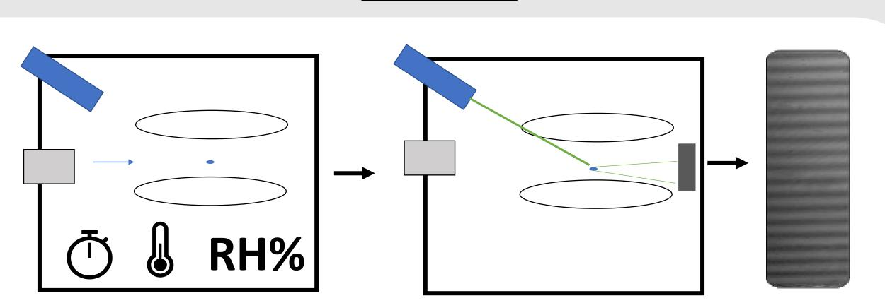
Bioaerosol of reproducible size are dispensed into the CK-EDB chamber, where one droplet is caught between electrodes. As the droplet equilibrates, it is interrogated by 523nm laser, with the scattered light providing an evaporation profile for particle size and phase morphology determined from the Fourier transform.
